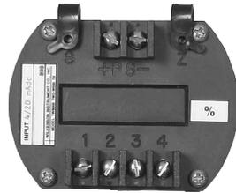
The TW8100 produces a DC output current proportional to its DC voltage or current input. A two-wire transmitter, its output regulates the current in a series loop while taking its operating power from the same current. Optional transformer input/output isolation is available.
