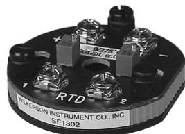
The SF1302 is a low-cost, reliable, RTD input two-wire transmitter designed with the OEM in mind. These transmitters are housed in a low profile, 50 mm diameter extruded aluminum case. This thin design allows two transmitters to be stacked in one standard connection head for use with dual RTD sensors.
