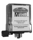
The MM4130 is used to provide output voltages or currents proportional to a thermocouple (T/C) input signal. The basic model MM4130 provides an output proportional to the millivolt signal from the thermocouple, while linearized model MM4130L corrects the thermocouple's nonlinearity to provide an output proportional to temperature. Both models provide cold-junction compensation via a solid-state sensor embedded in the thermocouple terminal strip.
