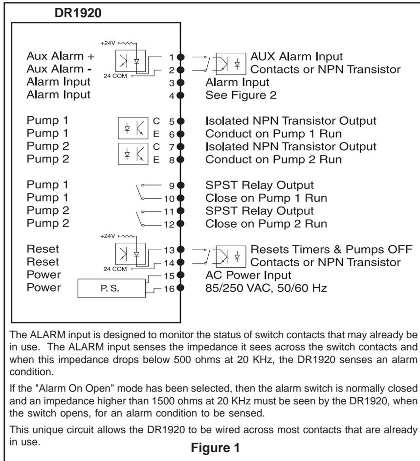
The circuit drawings below show how the DR1920 can be used to monitor contacts that are used to switch an AC relay and a DC relay with built in transient suppressor diode and LED status indicator.
