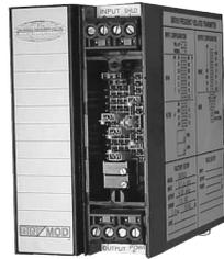
The DM7010 provides an isolated output voltage or current proportional to the frequency of the input AC voltage. The wide input voltage range allows the module to be used with low level magnetic pick-ups, for flow or speed applications, for digital signals, or for direct power line monitoring.
