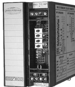
The *DM4130* provides an isolated output voltage or current proportional to the temperature as measured with a thermocouple. Any thermocouple may be used, and thermocouple types J, K, R, S, T, E and N can be linearized.
