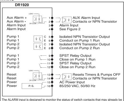
The ALARM input is designed to monitor the status of switch contacts that may already be in use. The ALARM input senses the impedance it sees across the switch contacts and when this impedance drops below 500 ohms at 20 KHz, the DR1920 senses an alarm condition.
